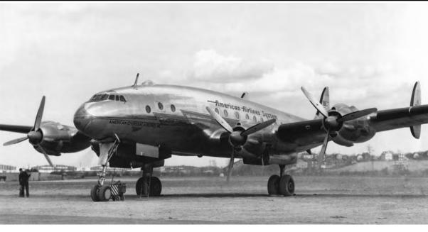
This Lockheed Constellation was the earliest version of the civilian Connie, the L-049. It can easily be distinguished from the later L-749 versions by the presence exhaust stacks the side of the NACA cowlings. The L-049 on photo, N90922 (2052) was delivered to American Air-Overseas lines 25 on March 1946 as
