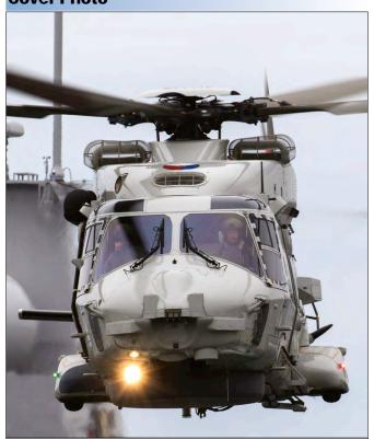
Sander Meijering captured N-233 during the Navy Days in Den Helder on 24 June 2017. This NH90-NFH is a de-scoped version, noticable by the missing FLIR, lack of sensor bulbs and missing cable cutter above the cockpit.
